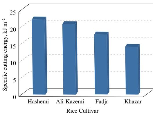
Figure 3. Specific cutting energy of cultivars at an identical test condition.
