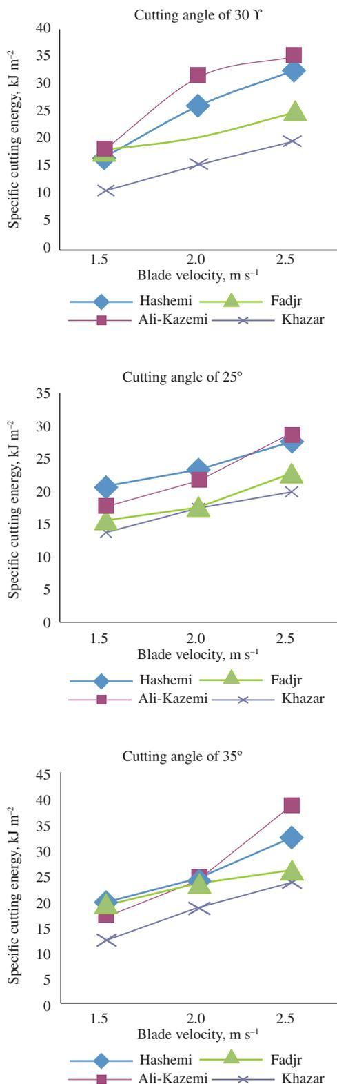
Figure 6. Specific cutting energy at different cutting angles.
