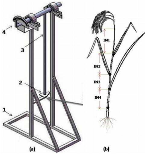
Figure 1. Schematic diagram of the pendulum displacement apparatus 1- Chassis; 2- Cutting blade; 3- Pendulum arm; 4- Angle pointer).
